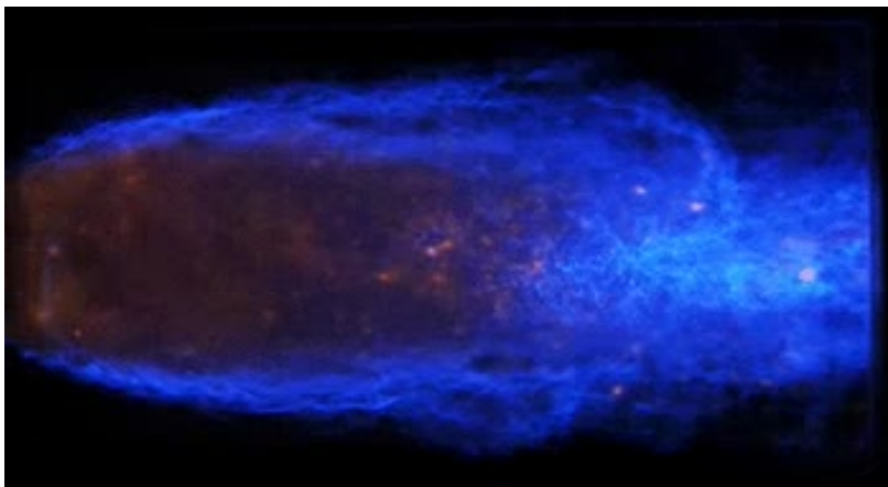
1 st place video 2018 “Violence - Thermo-Acoustic Combustion Instability in the Universal Bluff-Body Flame Experiment” Brendan Paxton (ISSI)
