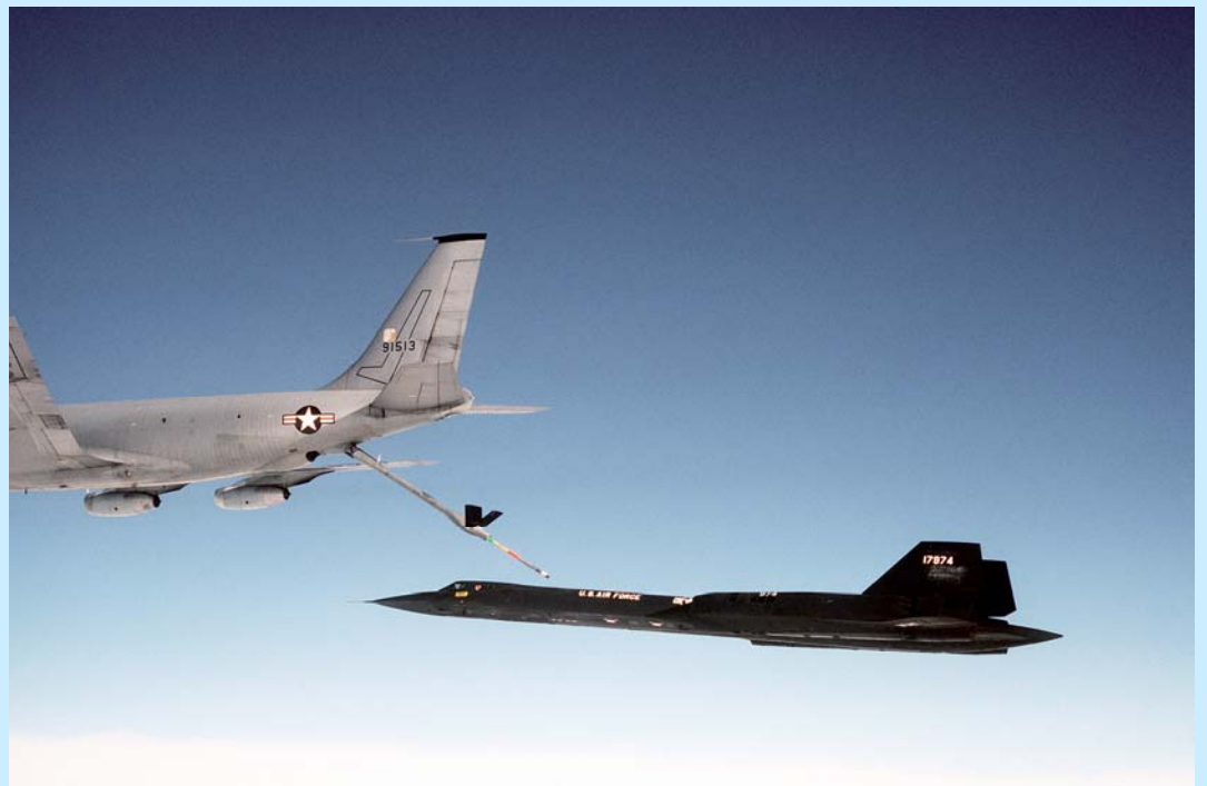
An SR-71 refueling from a KC-135Q Stratotanker Public Domain Image Courtesy of Wikipedia
